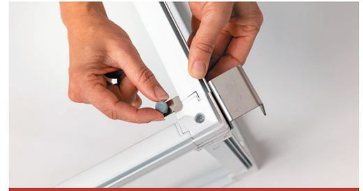
4. Close the clip with the screw for a secure connection.
