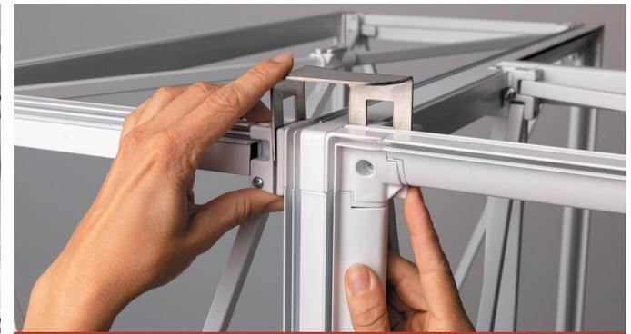
4. Slide the second connector in the slots of the hinges on top.
